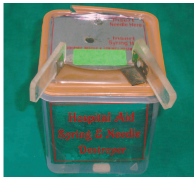
Fig. 20.8: Needle and syringe cutter and burner: An extremely versatile apparatus for incinerating the injecting needles and to cut the syringe, used in medical, dental surgery and surgical clinic. Health units, any where needles represent a likely risk of infection. The units in housed in an elegant casing and is a highly functional. Very efficient in operation. Specification: Voltage: 230 VAC at 50 Hz, Weight: 1.2 kg, Dimension: 180 × 163 × 132 mm
